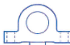
LWD-Low Wing Drilled
